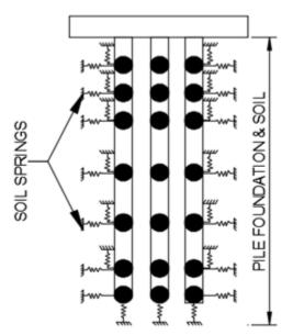
Figure 4. Spring represent interaction between soil and pile
