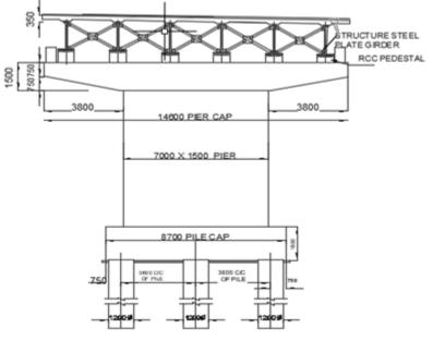
Figure 2. R. O. B Bent cross section
