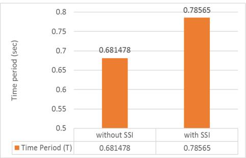
Figure 14 Comparison of the Time period without & with SSI
