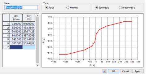
Figure 8. Force deformation function -Multilinear spring
