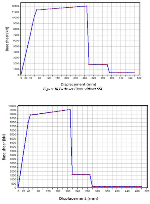
Figure 11. Pushover curve with SSI
