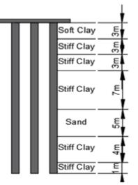
Figure 5. Idealized Soil profile for Bent Piles
